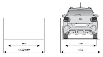
All measurements are in millimetres. \* Mirrors folded. \*\* With longitudinal bars.
